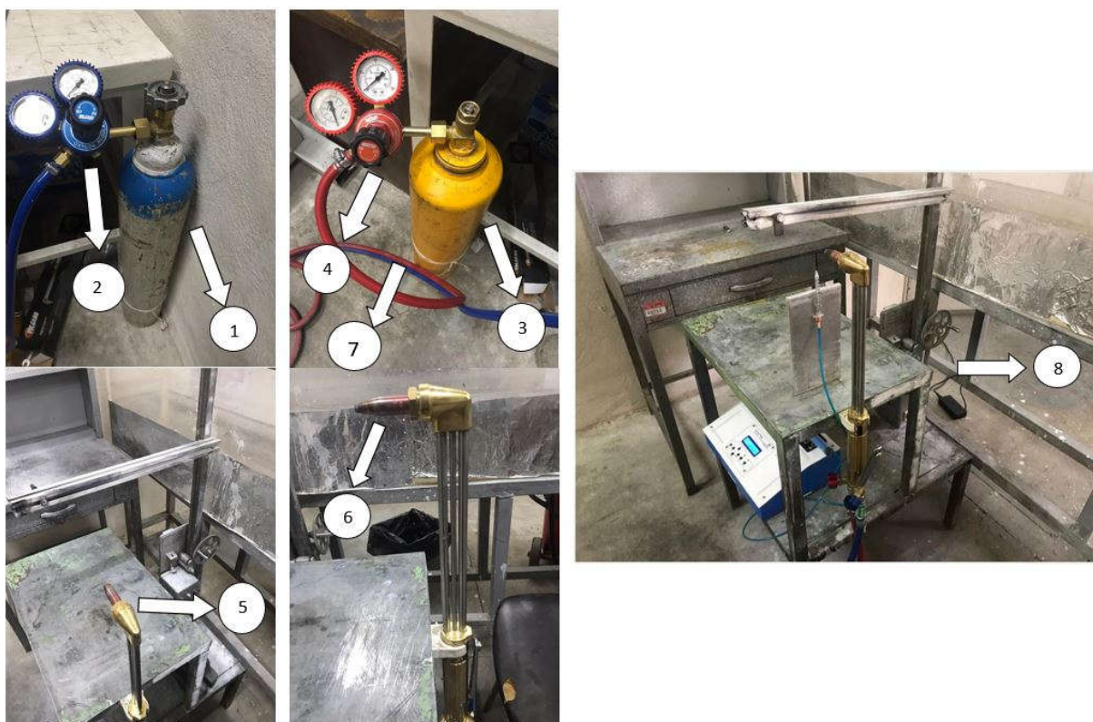
Figure 2: 1:Oxygen cylinder, 2: Oxygen manometer, 3: Acetylene cylinder, 4: Acetylene manometer, 5: Cutting Head, 6: Nozzle, 7: Hoses, 8: Operating mechanism
